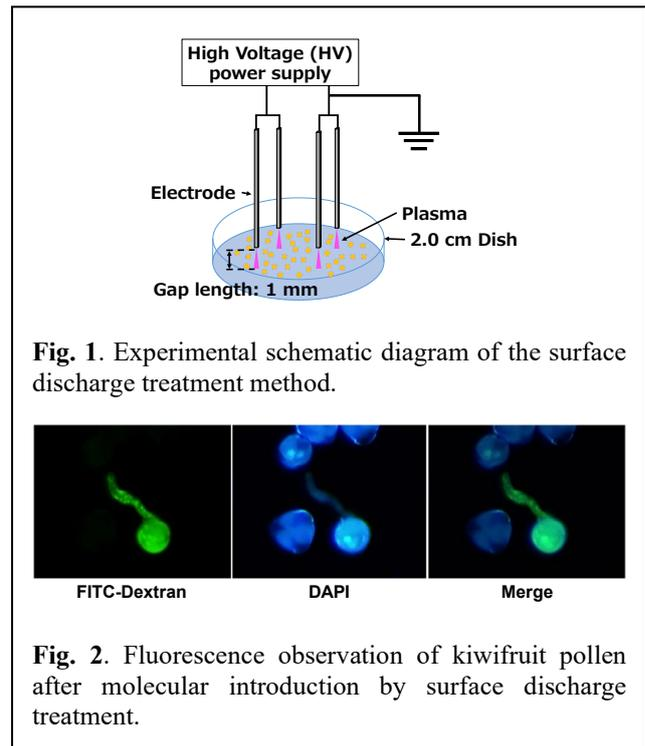
**Fig. 1.** Experimental schematic diagram of the surface discharge treatment method.
